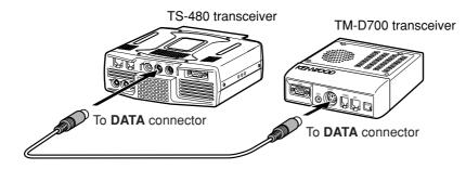
After connecting the 2 transceivers with the cable, access Menu No. 57 (DTS polarity) on the TS-480 transceiver and select "on". You will further need to adjust the audio input/ output level of the TS-480 transceiver using Menu Nos. 46 and 47.
