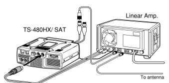
Use the supplied mini DIN (8-pin) connector to interface with the Linear Amp.
