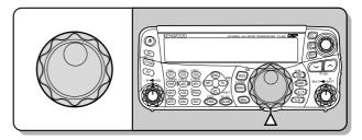
You may prefer directly entering a frequency using the numeric keypad if the desired frequency is far from the current frequency. Press **[ENT]**, then press the numeric keys as necessary. For details, refer to "Direct Frequency Entry" {page 34}.
