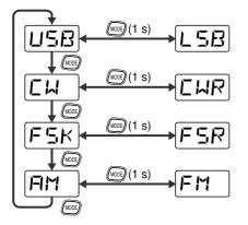
Access Menu No. 02 then press [~] to select "on" to turn the Auto Mode selection ON. When it is ON, "AUTO" appears. As a default setting, if you change the frequency above or below 9.5 MHz, the transceiver automatically switches modes; LSB for frequencies under 9.5 MHz and USB for frequencies equal to or over 9.5 MHz. You can further add the frequency table data to change the mode automatically {page 61}.
