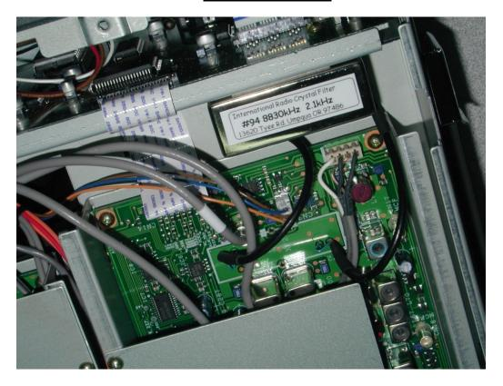
The INRAD #94 filter connects to the RF Board that is located on the radio bottom.
