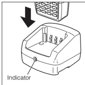
4. The red indicator turns off when the charge is completed. Remove the battery pack from the basket.
