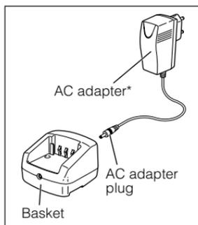
3. Mount the battery (with or without being attached to the unit) in the basket as shown. Turn off the unit while charging.
